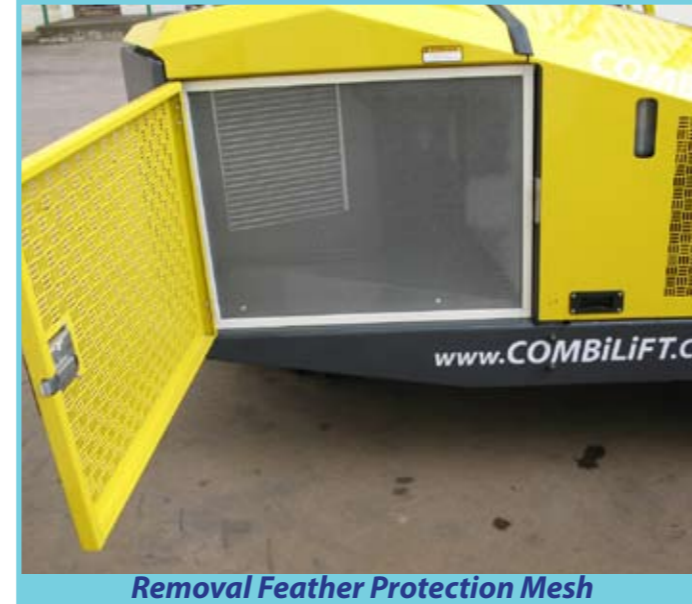
Removal Feather Protection Mesh
